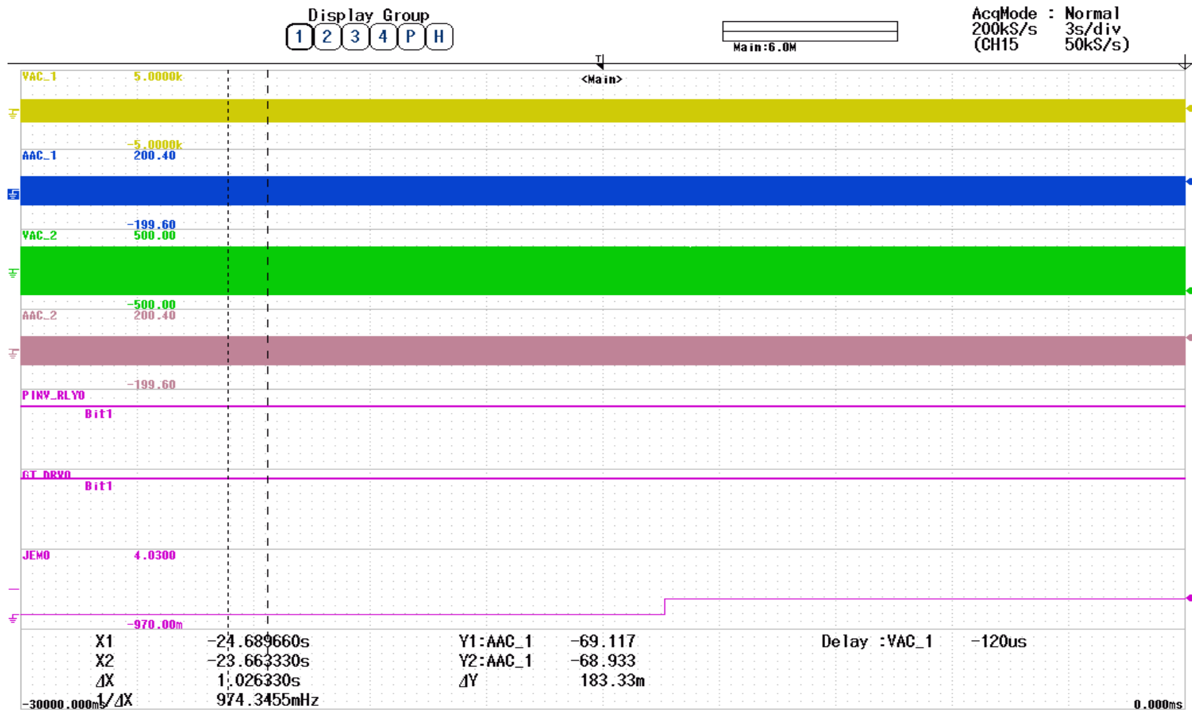
3.2.11.19: Scope- 3 rd harmonics=2.2V. JEM Status Standby to Active
