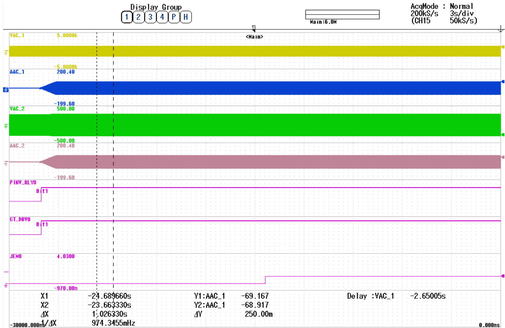
3.2.11.27: Scope-7 th harmonics=2.2V. JEM Status Standby to Active
