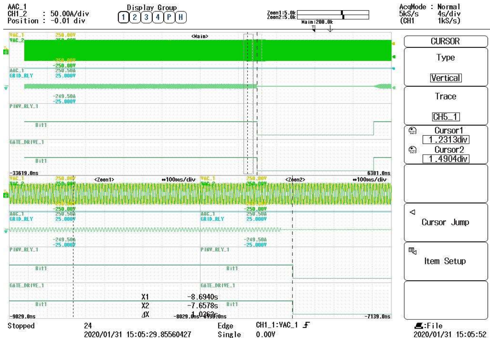
Figure 3.2.2.7 OFR Gate Block time = 1.026 sec (60.0Hz → 61.8Hz)
