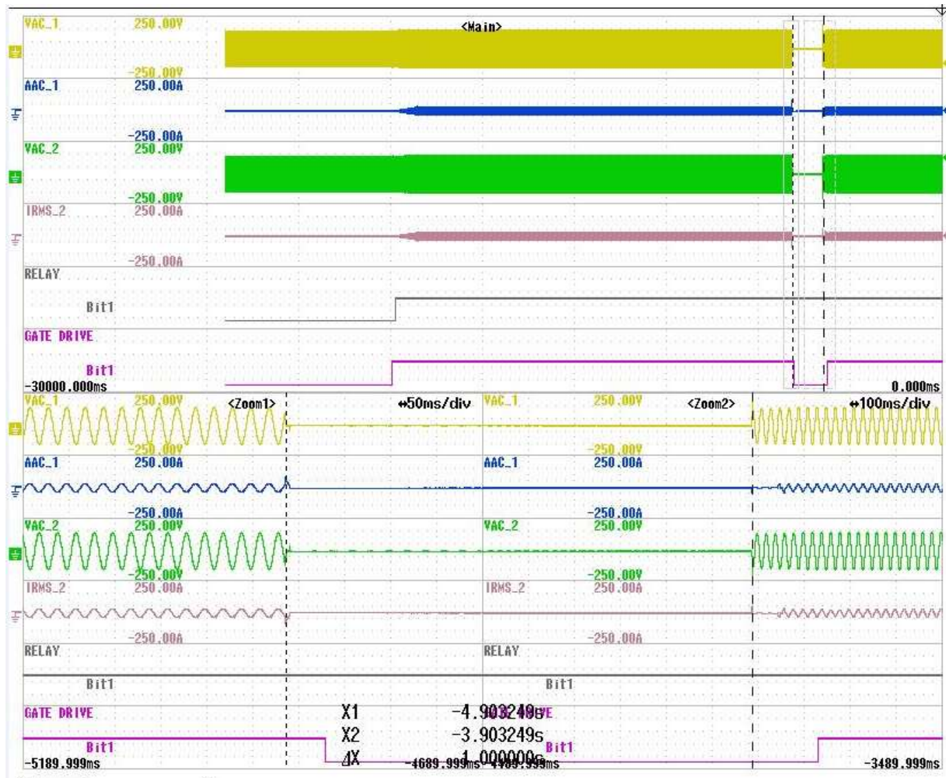
Figure 6.3.5 Instantaneous voltage drop at 45° entry angle (101Vrms → 0Vrms → 101Vrms)
