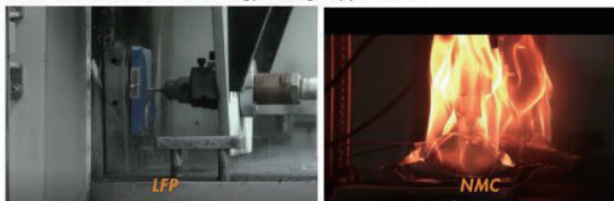
LFP and NMC nail-penetration testing comparison, LFP is only with smoke which NMC will be easily on fire and explosion
